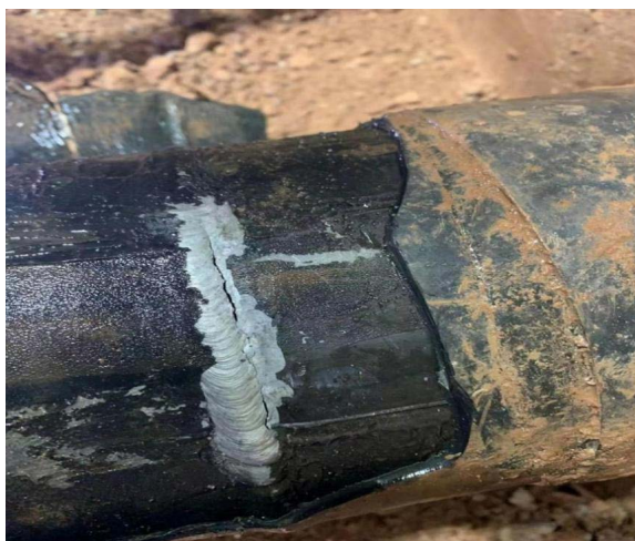
Figure 2. The picture of the welded crack on the scene 图 2. 现场焊口裂纹照片
