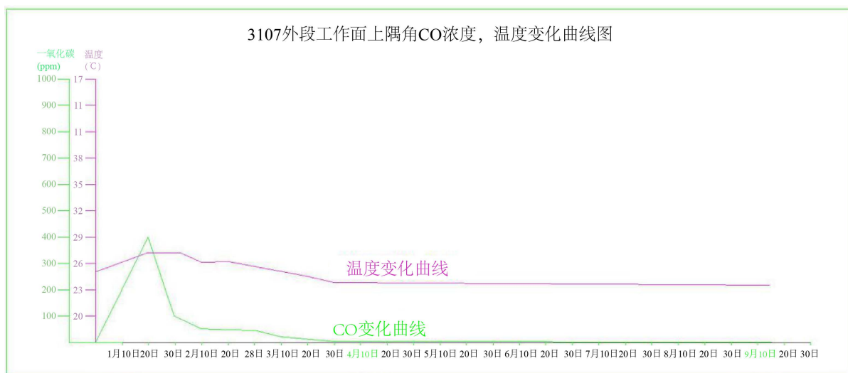
Figure 4. Curve of co concentration and temperature change at the upper corner of 3107 outer section working face 图 4. 3107 外段工作面上隅角 CO 浓度及温度变化曲线图
