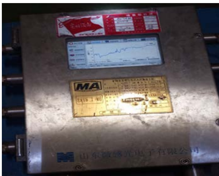
Figure 6. Temperature sensing optical fiber system
