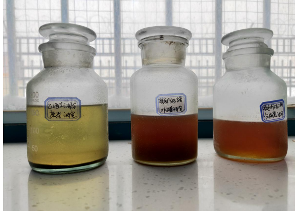
Figure 6. Oil freezing test 图 6. 油品冷冻试验
