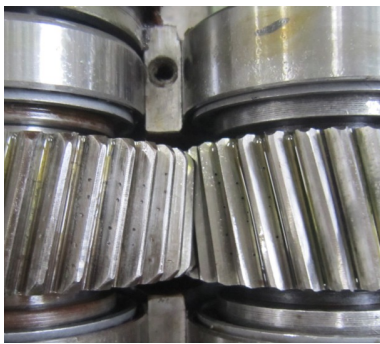
Figure 2. Pitting state of gearbox 图 2. 齿轮局部损伤(点蚀)示意图
