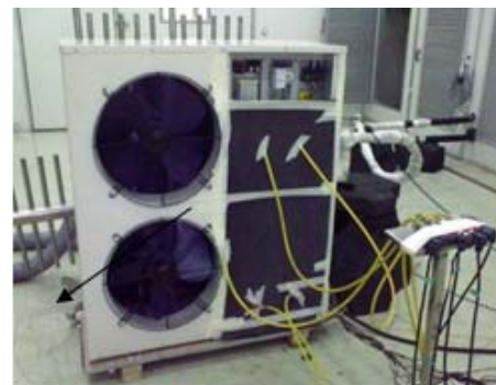
Figure 7. Testing pictures of HHP heat pump system 图 7. HHP 热泵机组测试图
