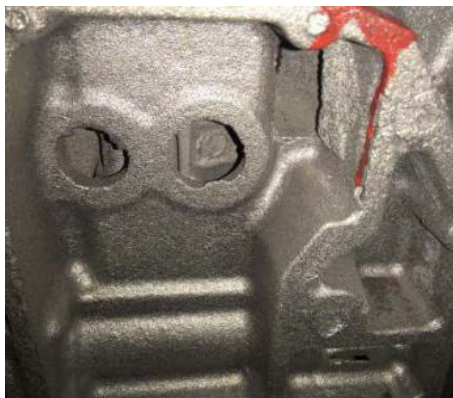
Figure 2. The avalanche sand of S2000 cylinder block
