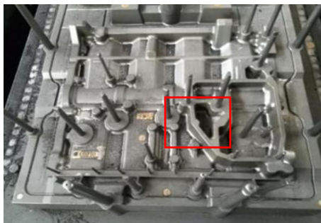
Figure 3. The abrasive shape mode of S2000 cylinder block
