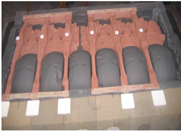
Figure 13. The down-casting core mode of K6000 cylinder block
