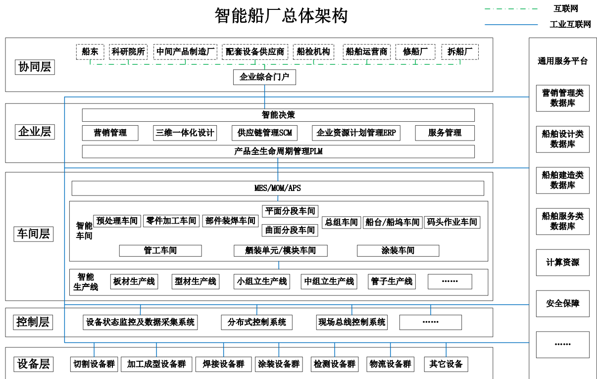
Figure 1. Schematic diagram of the overall architecture of intelligent shipyard
