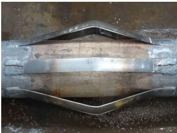
Figure 9. The state of the bow after expanded 图 9. 工具变径后扶正片的状态
