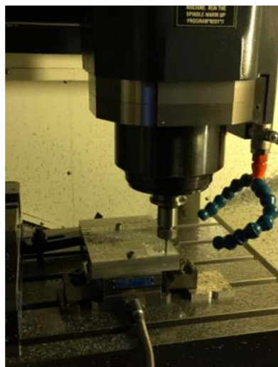
Figure 5. Machining test process of cam 图 5. 凸轮加工过程
