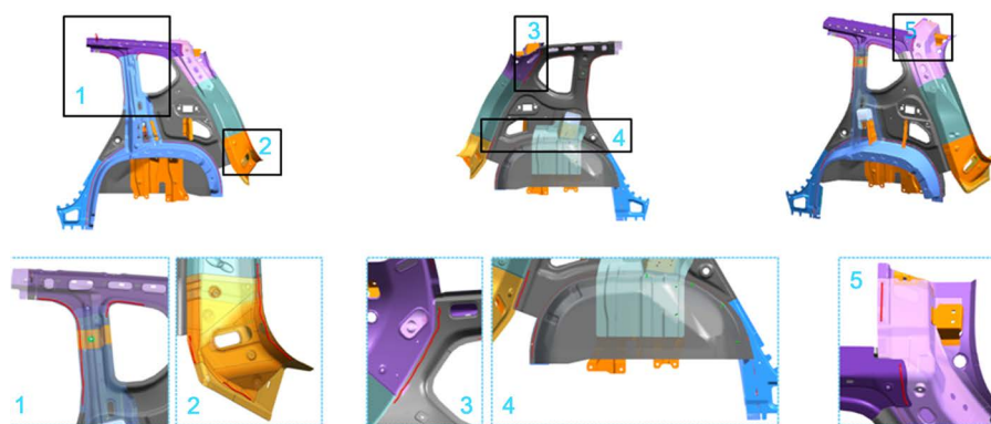
Figure 2. Coating position of structural adhesive on welded part of rearwall sidecover 图 2. 后侧围内焊合件结构胶涂布位置
