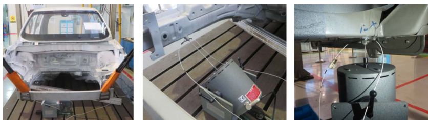
Figure 7. Position of excitation point in modal test of automobile white body
