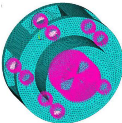
Figure 3. Flexible body model of the secondary planetary frame 图 3. 二级行星架柔性体模型
