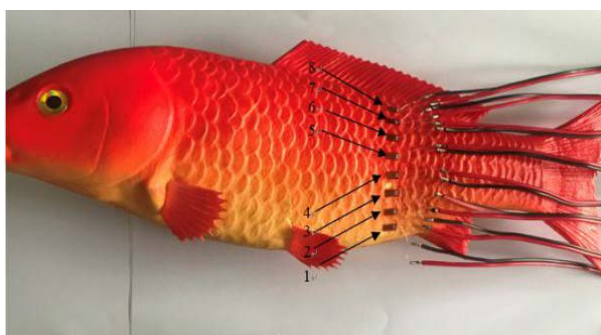
Figure 10. Strain gage paste physical photo 图10. 应变片粘贴实物图
