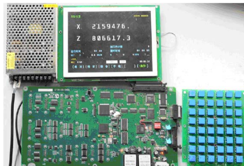
Figure 5. TDNC-SX system hardware platform 图 5. TDNC-SX 数控系统硬件平台
