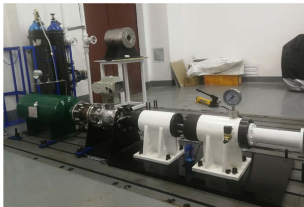
Figure 3. Physical picture of the main structure of the rapid compression machine 图 3. 快速压缩机主体结构实物图
