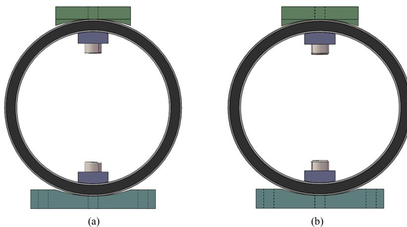
**Figure 1.** Vibration isolation ring composition. (a) Free state; (b) Locked state
