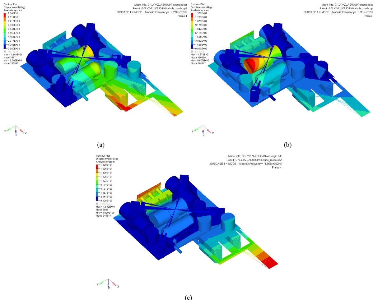
**Figure 6.** The first three-order modal formation of the refrigeration module locked by the unlocking device. (a) First-order mode; (b) Second-order mode; (c) Third-order mode
