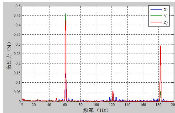
**Figure 7.** Translational excitation force amplitude curve
