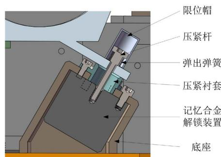
**Figure 2.** Schematic diagram of the structure of the unlocking device in the compressed state
