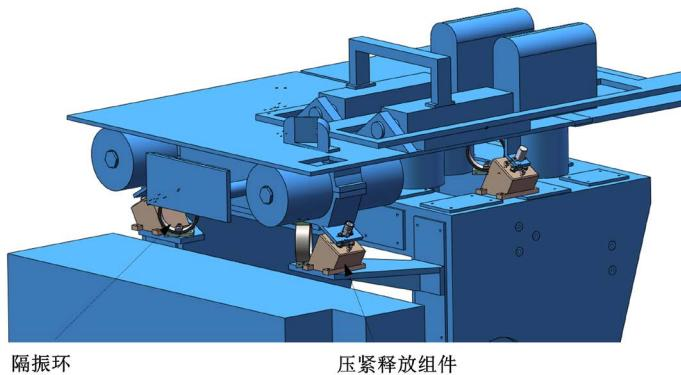
**Figure 4.** Vibration isolation unlocking device system scheme
