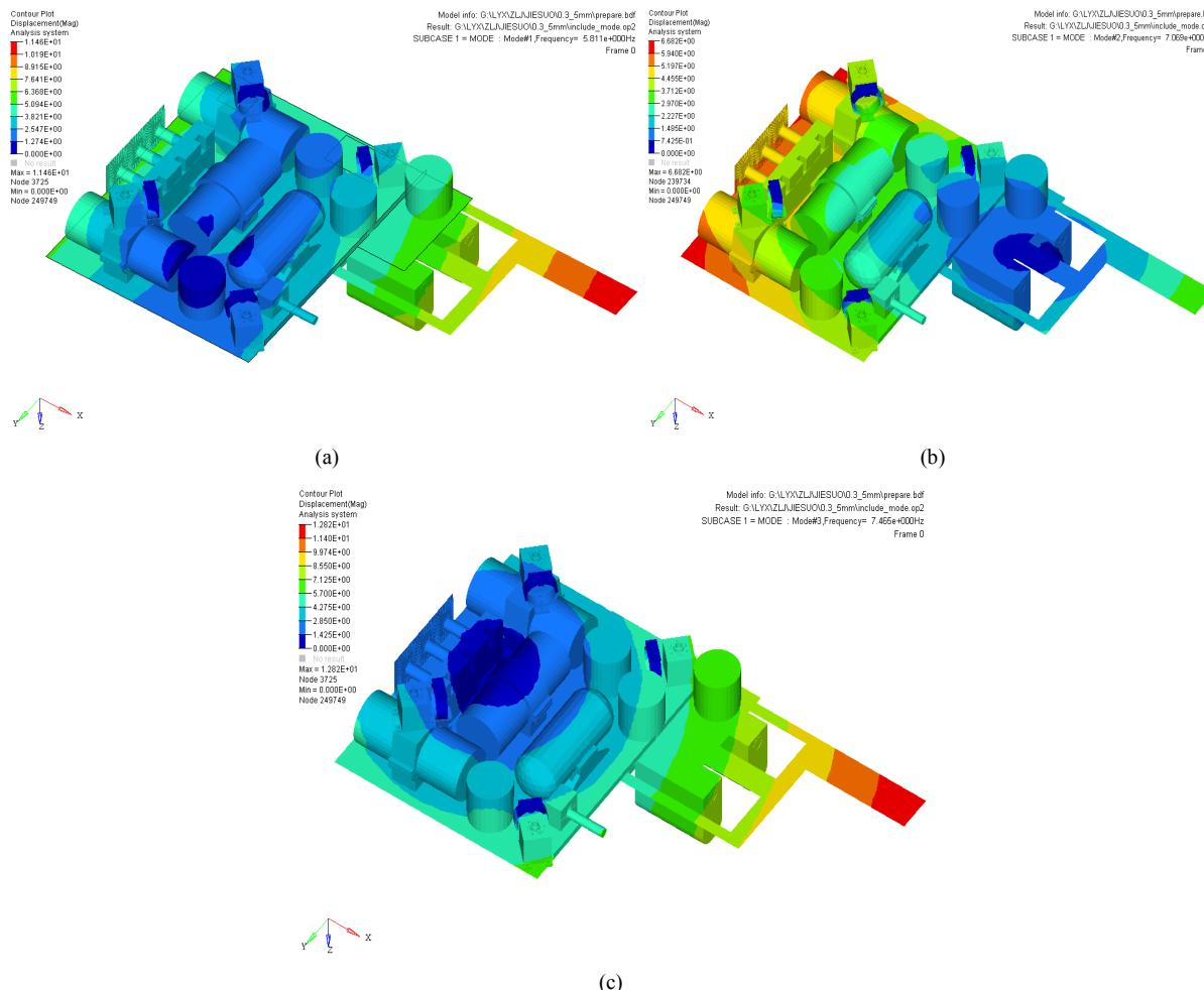
**Figure 5.** The first three-order modal array of the refrigeration module after installing the damping ring. (a) First-order mode; (b) Second-order mode; (c) Third-order mode
