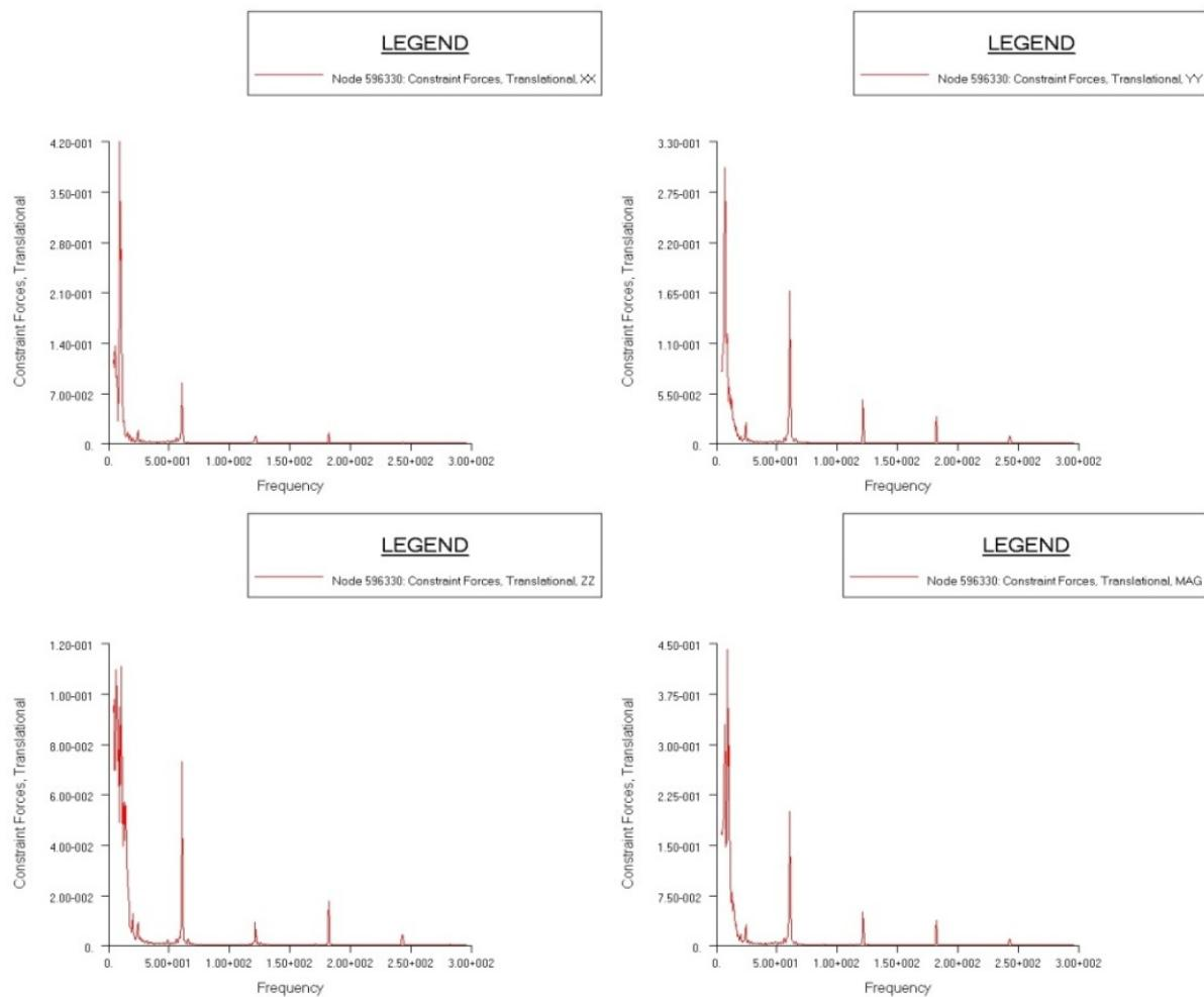
**Figure 8.** The output curve of the reaction force at the common restraint position of the vibration isolation ring
