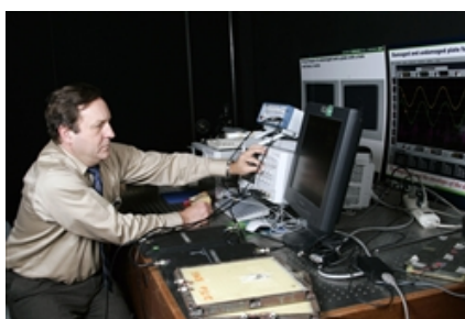
Figure 7. Ultrasonic testing of crack in shaft assembly
