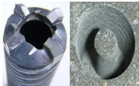
Figure 4. Revision B (left), the completed basalt sample (right)
