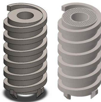
Figure 7. Before replacing the steel body of the drill bit (left), after replacing the lattice structure (right)
