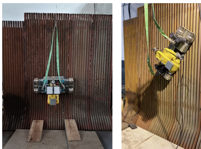
Figure 7. The wall climbing robot moves on the water wall vertically (left) and horizontally (right)
