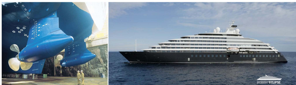
Figure 1. Scenic Eclipse and the Azipod type thruster system
