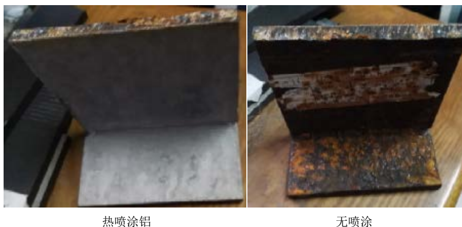
Figure 13. Comparison of morphology of 72-hour salt spray test samples 图 13. 72 h 盐雾试验试样形貌对比
