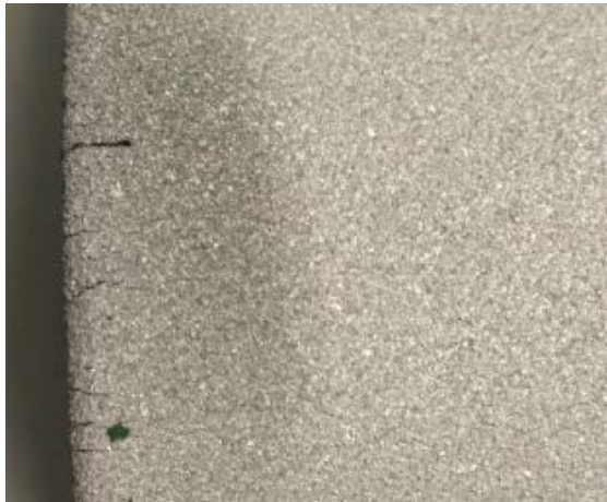
Figure 8. Bending specimen 1 cracking state 图 8. 弯曲试样 1 开裂状态
