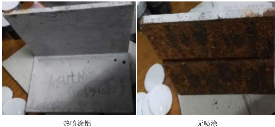
Figure 14. Comparison of morphology of 500-hour salt spray test samples 图 14. 500 h 盐雾试验试样形貌对比
