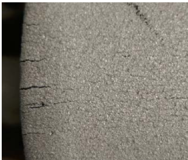
Figure 12. Bending specimen 3 cracking state 图 12. 弯曲试样 3 开裂状态
