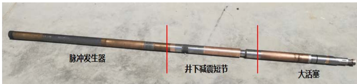
Figure 5. Downhole damping stubs (hydraulic shock absorbers)
