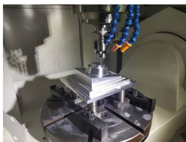
Figure 22. On-machine measurement process of feature workpiece 图 22. 特征工件在机测量过程
