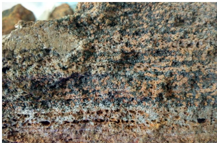
Figure 2. Photograph of ring sample in Rotary kiln
