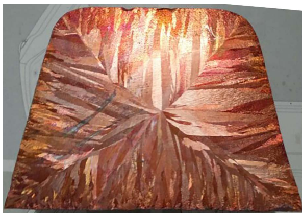
Figure 4. Low magnification microstructure 图 4. 铸坯低倍组织
