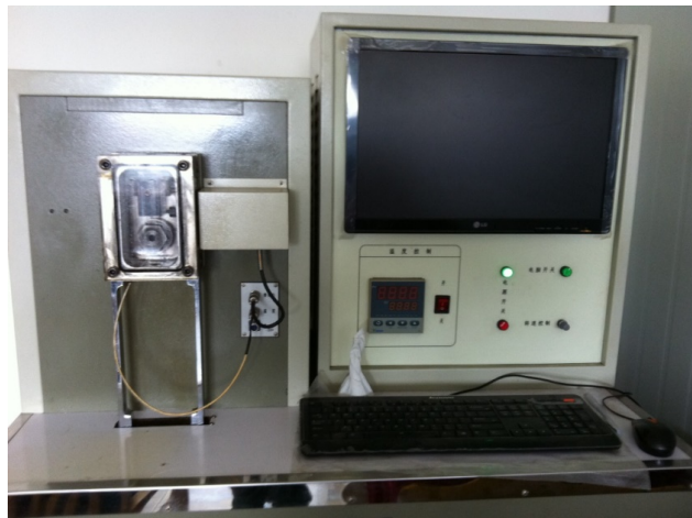
Figure 1. MRH-3G high speed ring block friction and wear test machine 图 1. MRH-3G 屏显式高速环块摩擦磨损试验机
