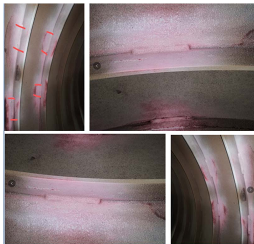
Figure 4. Dye detection of welds between inner surface of cylinder and stiffener 图 4. 筒体内表面与加强筋的焊缝着色探伤
