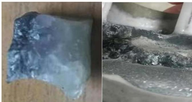
**Figure 4.** The sample 1.5 V negative (left side) and 4.5 V negative (right side)
