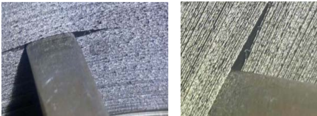
Figure 1. The photo of edge crack 图 1. 边裂缺陷照片
