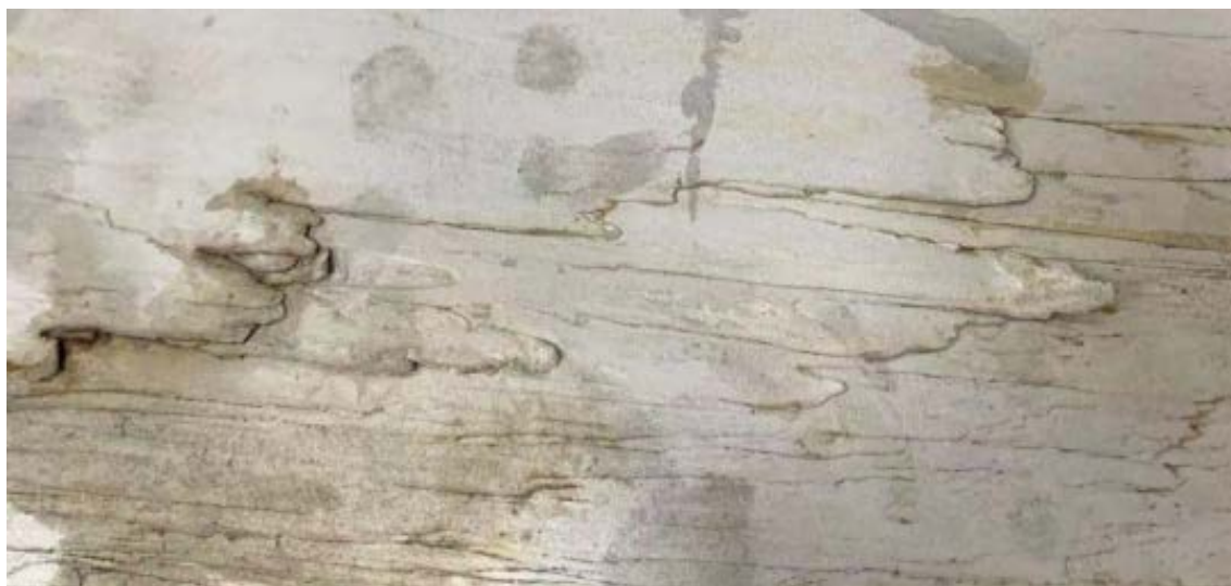
Figure 1. Surface peeling sample of hot-rolled pickling plate
