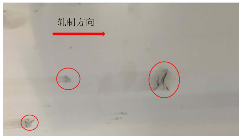
Figure 5. Surface crack morphology of cold rolled sheet 图 5. 冷轧板表面裂纹缺陷形貌
