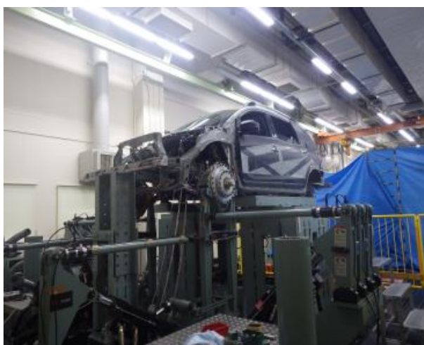
Figure 3. BIW fixed fixtures
