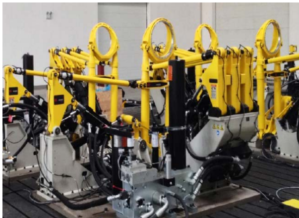
Figure 1. MTS 329PC 6-DOF spindle-coupled road simulation test bench
