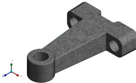
Figure 2. Finite element model of steering arm
