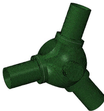
Figure 3. Schematic diagram of grid model of wind turbine axle 图 3. 涡轮机轮轴的网格模型示意图
