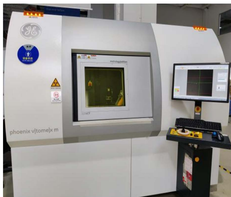
Figure 3. Pheonixv X-ray computed tomography system 图 3. Pheonixv X 射线计算机断层扫描系统
