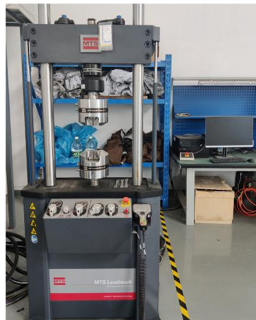
Figure 2. MTS Landmark Electro-hydraulic servo dynamic test system
