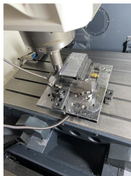
Figure 2. Milling process of aluminum-based silicon carbide 图 2. 铝基碳化硅铣削过程
