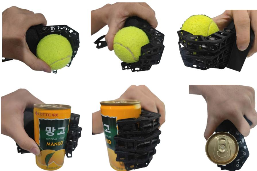
Figure 14. The prosthetic hand allows for an adaptive grip
