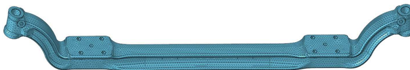
Figure 2. Front axle finite element model
