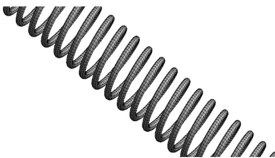
Figure 7. Meshing of finite element model of reset spring 图 7. 复位弹簧有限元模型网格划分
