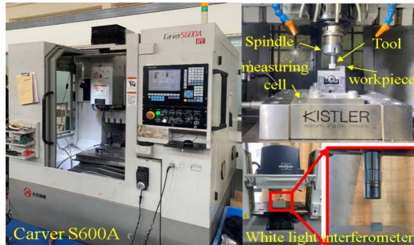
Figure 3. Test equipment and site settings 图 3. 试验设备及现场设置
