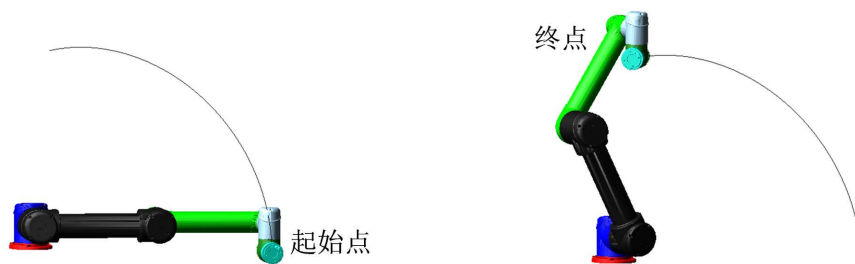
Figure 6. Quintic polynomial programming driven end-effector trajectory 图 6. 五次多项式规划驱动末端轨迹
