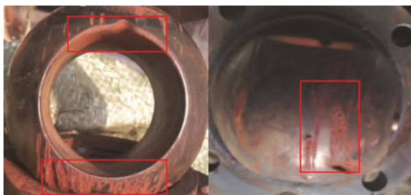
Figure 5. Physical image of erosion and wear
