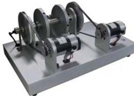
Figure 9. Experimental verification platform of the DC servo system 图 9. 直流伺服系统实验验证平台
