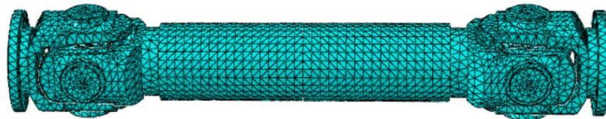
Figure 3. Cross shaft universal coupling mesh model
