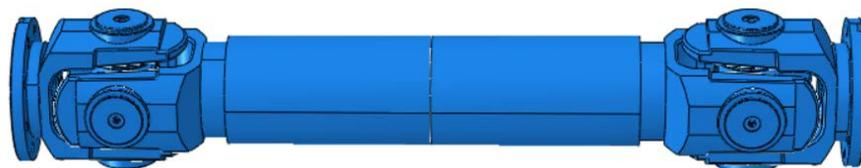
Figure 2. Cross shaft universal coupling finite element model
