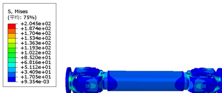
Figure 5. Maximum stress clouds for cross shaft universal couplings
