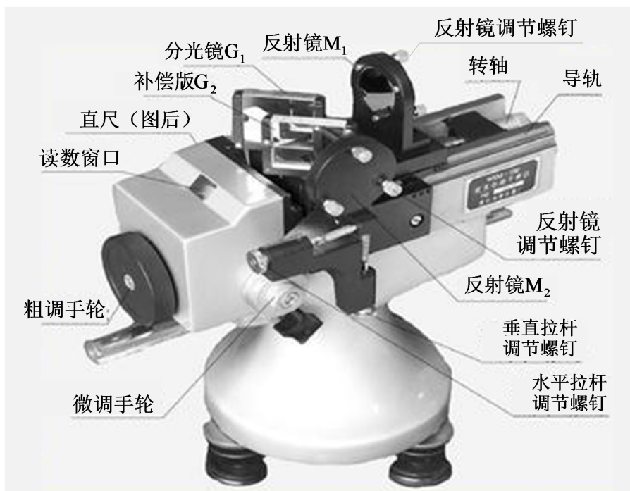
Figure 6. Michelson interferometer 图 6. 迈克尔逊干涉仪
