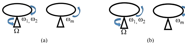
Figure 1. Model of the rotating optomechanical system, (a) the cavity is driven from its left side; (b) the cavity is driven from its right side
