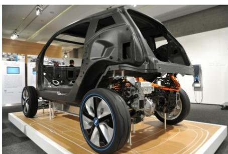
**Figure 2.** Carbon fiber frame of BMW i series
