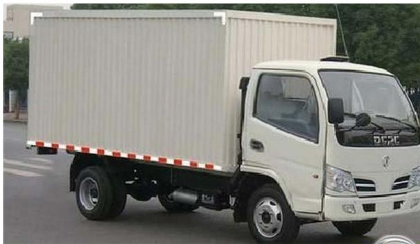
**Figure 5.** The truck with composite box
