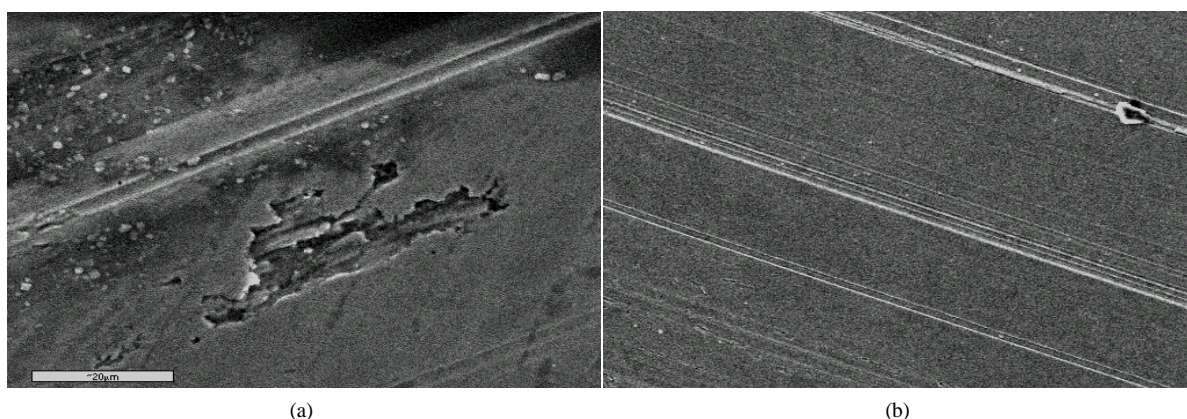
Figure 2. Nano-diamond lubricants can greatly reduce surface roughness of friction pairs; Abrasion test conditions: load = 150 N, sliding speed = 1.83 m/s, sliding distance = 6594 m; Comparison of surface morphology of steel/steel friction pair; (a) Spindle oil; (b) Spindle oil + 0.025% nD
