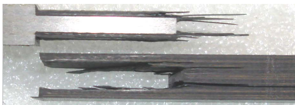
Figure 6. Typical failure state at 60 kN fatigue peak load
