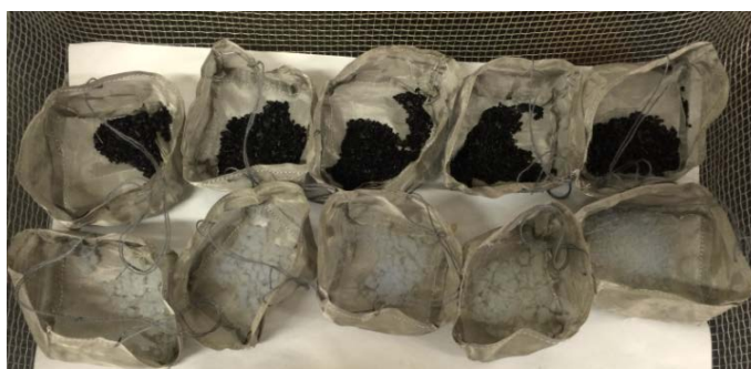
Figure 1. String bag made with stainless steel wire mesh 图 1. 丝网网兜(黑色为活性炭, 白色为硅气凝胶)
