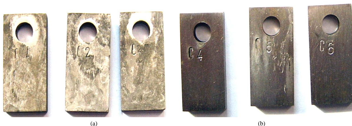
Figure 1. Corrosion morphology of X52 steel in H 2 S/CO 2 simulated water system: (a) gas phase; (b) liquid phase 图 1. X52 钢在 H 2 S/CO 2 模拟水体系中的腐蚀形貌: (a) 气相; (b) 液相
